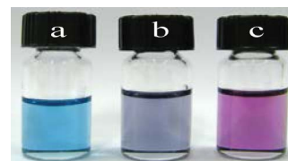
Fig. 2 Color changes of complex 1 upon addition of various anions in DMSO/H 2 O (4/1, v/v): (a) 1 only; (b) 1 + 2.0 equiv. of L-aspartate; (c) 1 + 2.0 equiv. of D-aspartate.
